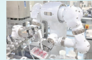
Human-type robot for general-purpose experiments "Maholo"
